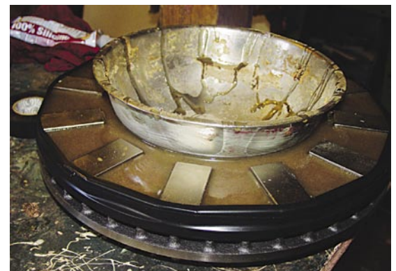
Photo 10: Molding the magnet rotors requires a stainless steel mixing bowl at the center and some duct tape around the edge to hold the resin.
