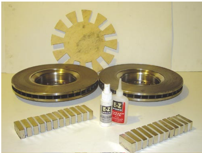
Photo 8: Magnet rotor materials include a plywood jig, two brake rotors, 24 magnets, and cyanoacrylate glue.
